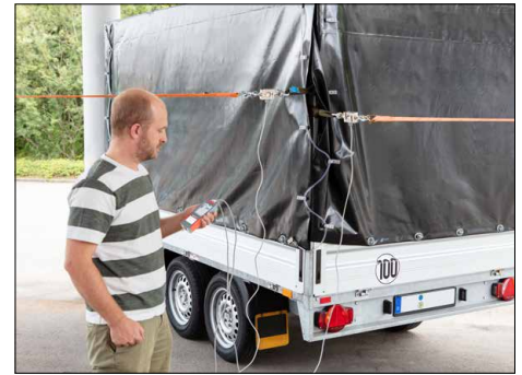
Measurement of forces in different tensile or compression directions possible with only one measuring device
