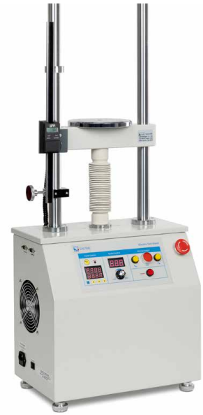
Motorised test stand incl. length measuring device LB
