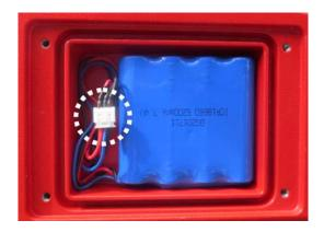
Before the first use, the rechargeable battery should be charged by connecting it to the mains power cable for at least 24 hours. The operating time of the rechargeable battery is approx. 60 hours.
