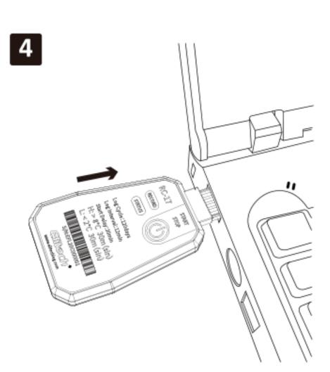
Insert the recorder into the USB port of the computer to view the PDF data report
