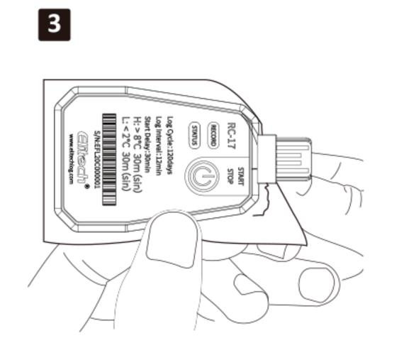
Press and hold the button for 5 seconds to stop recording, the red light flashes 5 times, tear open the plastic bag, reveal the USB interface
