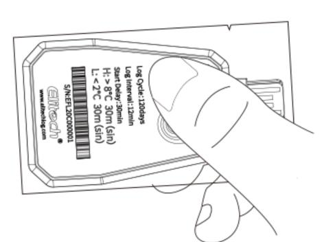
Long press for 5 seconds to start recording, the green light flashes 5 times
