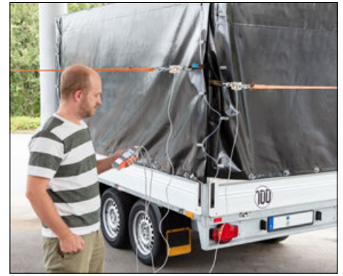
Measurement of forces in different tensile or compression directions possible with only one measuring device
