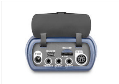
... and data transfer using MicroSD (4G) memory card (included in delivery), RS-232 or USB
