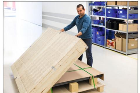
**1** Weighing plate can be unscrewed - The weighing plate can be conveniently unscrewed for maintenance or cleaning purposes
