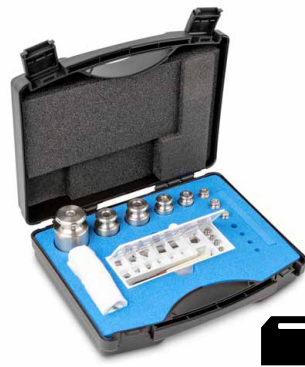
Plastic case, lined, for weight sets, knob shape, finely turned stainless steel
