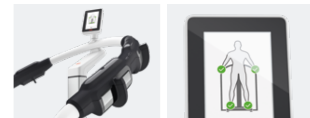
The illuminated footprints embedded in the glass platform show patients exactly where to stand. The display immediately indicates whether the electrodes have made contact and the measurement can start.
