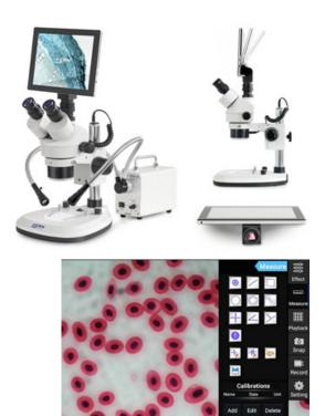
Integrated software with measuring function
